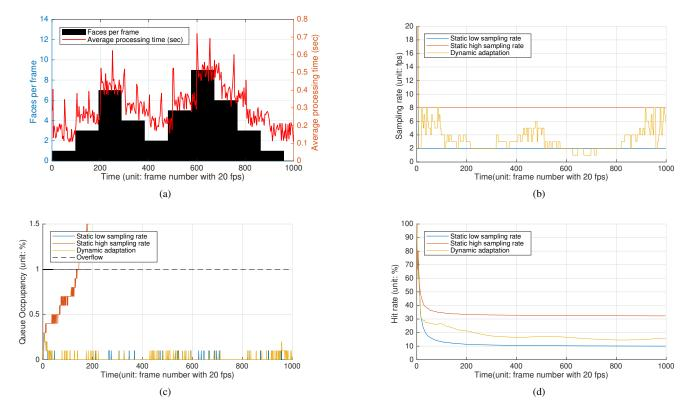
Fig. 3. Data-intensive performance evaluation results of sampling rate adaptation with (8). Fig. 3(a)–(d) show the performance evaluation results depending on various criteria such as sampling rate dynamics, queue stability, and hit ratio which is represented by the percentage of cumulative sampled image over total frames respectively as time elapsed: (a) Scenario, (b) changes in sampling rate, (c) stability of the queue, and (d) hit rate.
