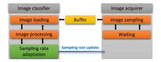
Fig. 1. Improved pipeline of the real-time computer vision system with the additional procedure that computes optimal sampling rates and adjusts the values.
